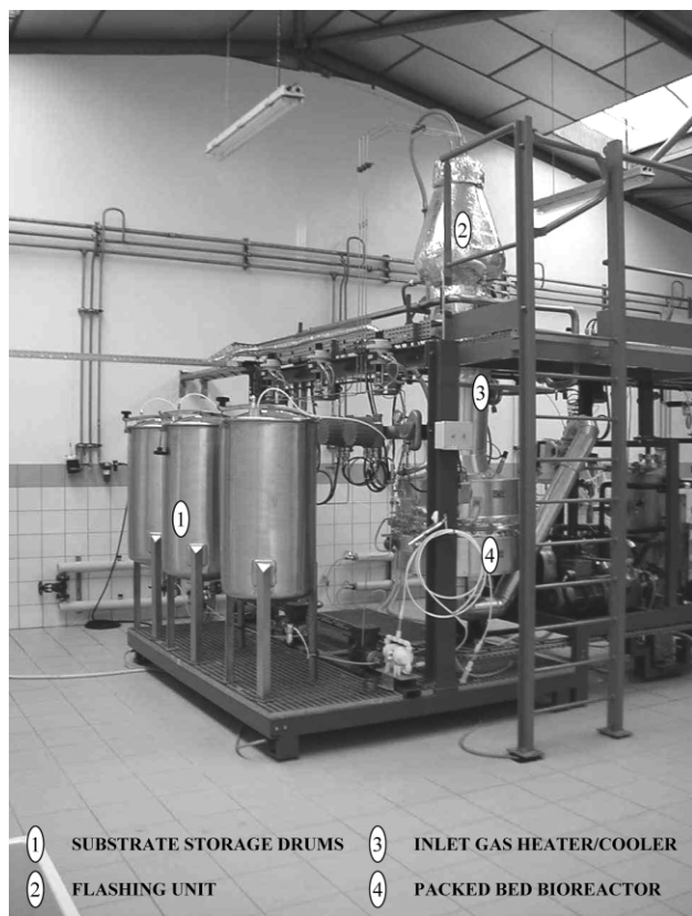
Fig. 10 Industrial solid-gas bioreactor (University of La Rochelle).
